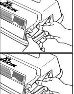
Remove the belt from the brush roll pulley and the motor drive shaft.
